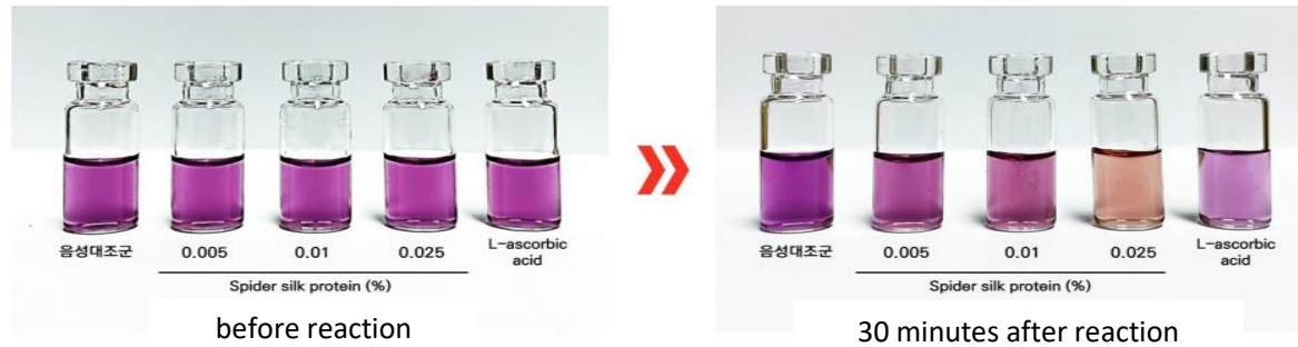
Figure 3. Color change image of DPPH free radical scavenging ability of test substance Spider silk protein'.
